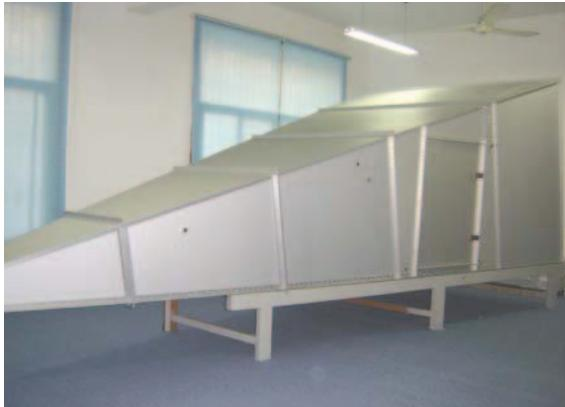
Figure 13 Photo of GTEM cell.
